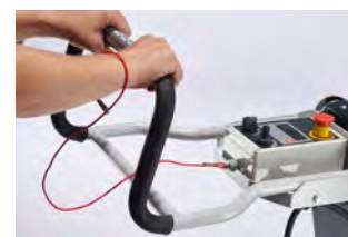
Dead man's switch for safe working
