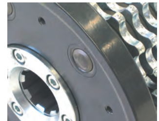
Drum with replacement bushes = longer service life
