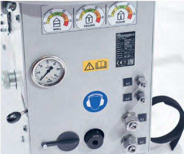
Setting of contact pressure and hydraulic connections
