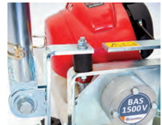
Fixation screw for angle adjustment
