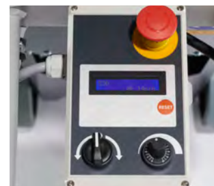
Display with power display and operating hours counter
