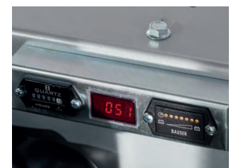
Display for battery and operating hours
