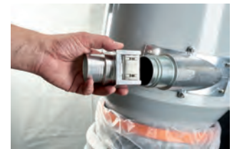
With click system for suction hose attachment
