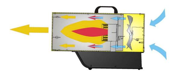
The "LPG" hot air generator is characterized by the total use of the fuel, by heat exchange due to direct mixing of the intake air and the combustion products. Safety devices always guarantee the correct operation of the machine. The accurate selection of materials ensures high reliability, while the noise impact has been reduced to minimum. It has a pratical handle for easier transport and handling. The appliance is manufactured in compliance with the EN 1596 Standard.
