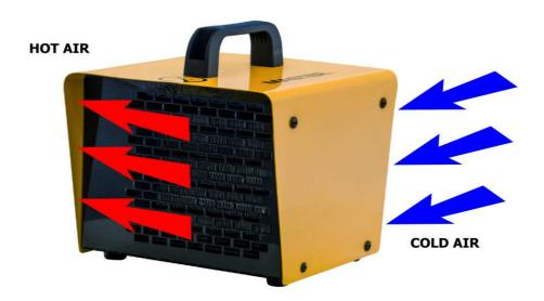
The device works on the principle of forced convection. The airflow is forced by fan. The cold air is sucked in at the rear of the unit. The cold air becomes heated when flow through the PTC heating element. The heated air exits the front of the heater. The device can heat a half or full power. The device is equipped with thermal protection running automatically. The device has a thermostat for adjusting temperature in the range 0°C - 40°C.
