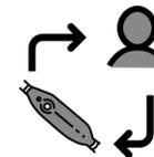
The PRCD system (protective residual current device) is optional. This system immediately disconnects the machine if there is a current leakage of 10mA. This is an additional protection available for the user and for the equipment.
